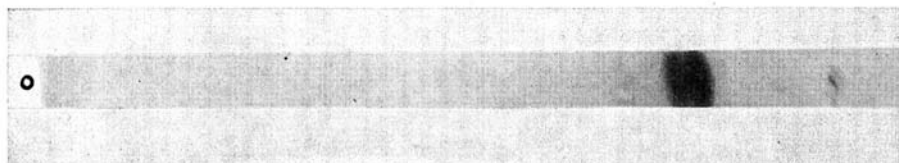
Fig. 2. Starch-gel electrophoretic pattern of a fraction obtained from carboxymethyl cellulose separation of wheat globulins.
