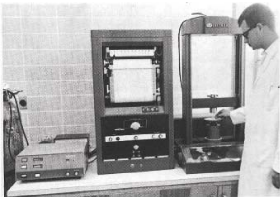
Fig. 1. Instron Universal Tester (Type T.M.) equipped with a special "tooth" used in firmness measurements of cooked spaghetti.
