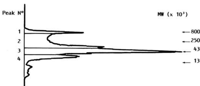
Fig. 1. Size-exclusion high-performance liquid chromatography elution curve of sodium dodecyl sulfate-phosphate buffer extract of durum wheat, cultivar Kidur.
