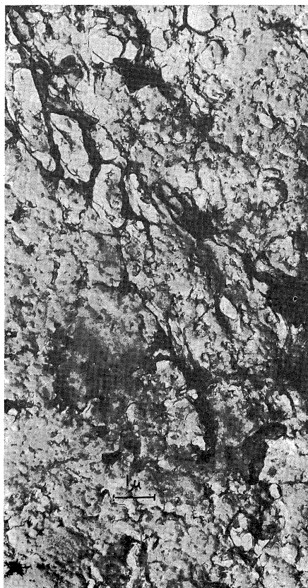
Fig. 5. Shadowed carbon replica of the surface of stretched unmodified crude gluten.
