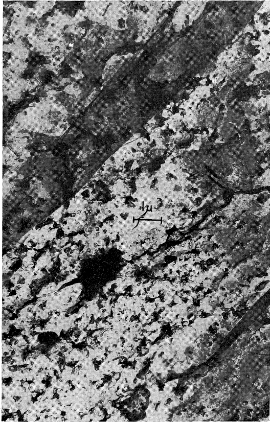
Fig. 7. Shadowed carbon replica of the surface of stretched 44% acetylated crude gluten.
