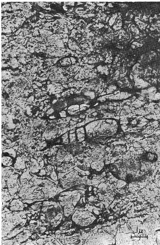
Fig. 6. Shadowed carbon replica of the surface of stretched 36% methylated crude gluten.
