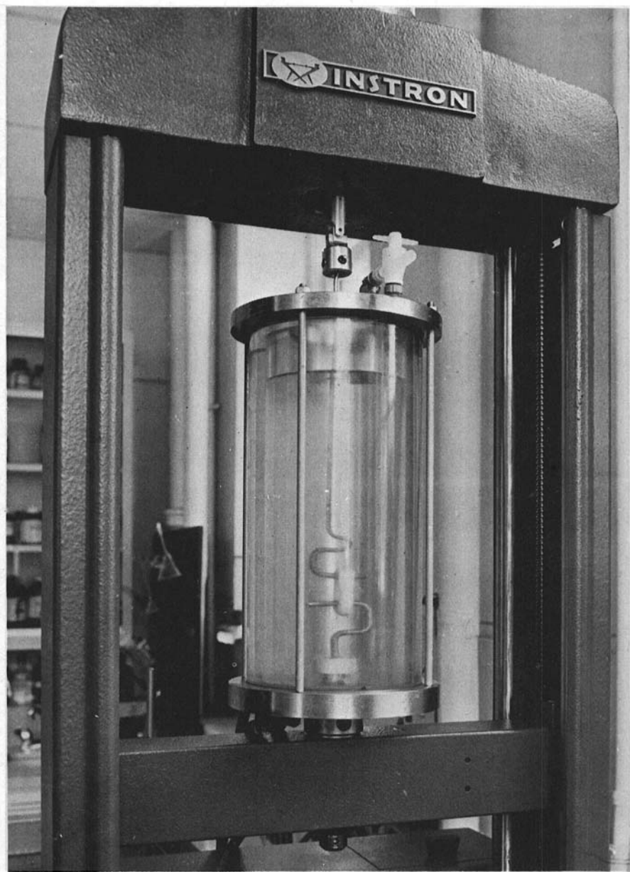
Fig. 1. Cross-head attachment of the Universal testing machine (Instron) for stretching dough rings in simple tensile mode while submerged in buoying liquid of matching density.
