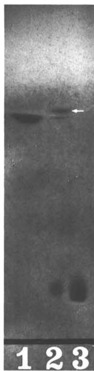
Fig. 3. Thin-layer chromatogram of lysophosphatidyl ethanolamine (1), electroextracted phospholipids in wheat prime starch granules (2), and lysophosphatidyl choline (3). Developed on thin-layer chromatography plate cellulose F (Merck) with chloroform/methanol/water (65:25:4, v/v) and detected by Dittmer reagent. Arrow indicates bromphenol blue.
