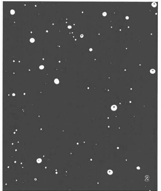
Fig. 2. Light micrograph of isolated starch 24 days after flowering photographed with darkfield microscopy showing high contrast useful for image analysis ( \times 112.5 ).
