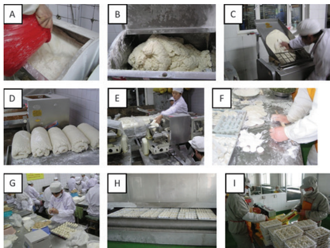
Fig. 2. Commercial processing of jiaozi . A , Salt solution is added to flour; B , dough is rested inside the mixer; C and D , dough is sheeted a few times, followed by resting to relax the gluten network; E , dough is divided into small dough pieces using a divider; F and G , jiaozi wrappers are formed by hand-rolling; H and I , jiaozi is frozen and packaged for market.
