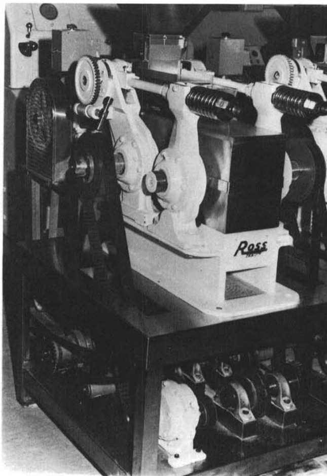
Fig. 1. The first break rolls of the Grain Research Laboratory 10-in. (254-mm) laboratory research mill.
